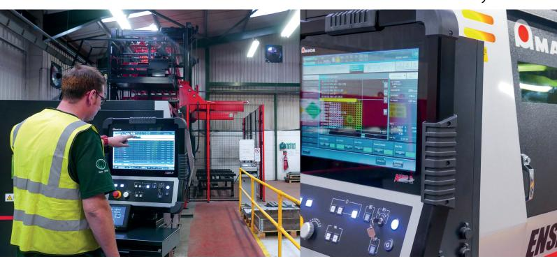
Greenfield Engineering, a market leader in precision sheetmetal fabrication, has invested in an AMADA ENSIS-3015AJ 3 kW fibre laser with AS LUL automation tower. Saving on the previous cost of outsourcing laser work, the machine is the first in the UK to feature AMADA's OVS system, which allows pre-punched and formed sheets to be loaded on the ENSIS for laser cutting.
