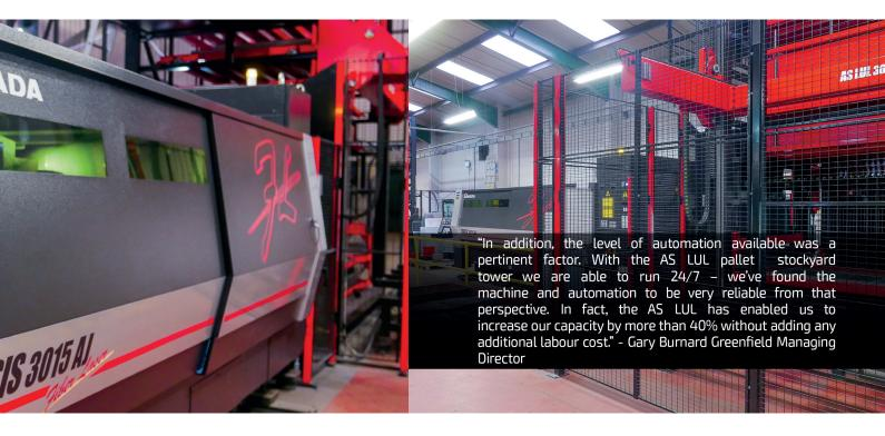
"OVS allows us to take punched parts and put them on our ENSIS-3015AJ, which verifies the position of two punched datum holes and automatically adjusts the laser program to compensate for any inaccuracies in sheet loading," explains Mr Burnard. "We thus end up with combined process parts without the need or cost of a punch-laser combination machine."
